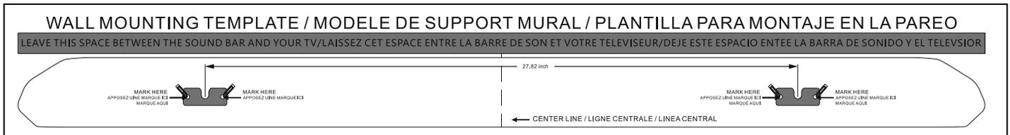
Place the included wall mounting template against the wall under your TV. Mark the four bracket holes using a pencil.
